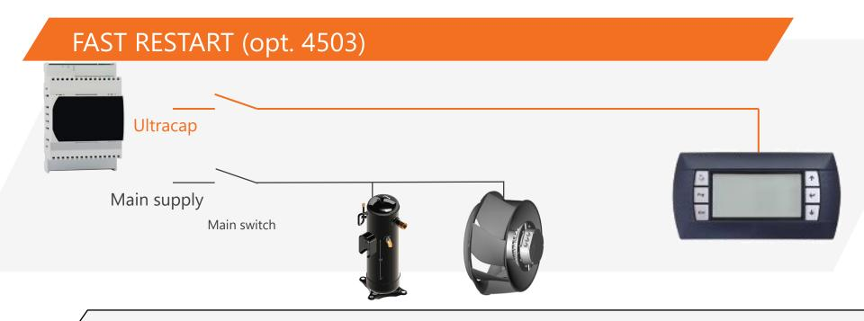
In the event of brief blackouts, it keeps the unit's microprocessor powered for a few minutes and ensures the **rapid resumption** of machine operation when normal power supply conditions are restored.
