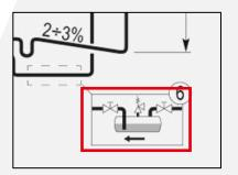
In those installations with equivalent lengths of refrigerant lines more than 25 m (up to 100m), the installation of an additional liquid receiver is recommended, to be installed on the liquid line outside the unit (by the installer).
