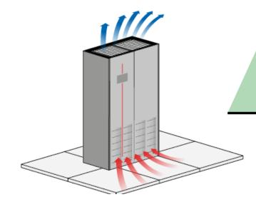
**OVER** air flow delivery and return from the **front**. Ideal for data centers without raised floor.
