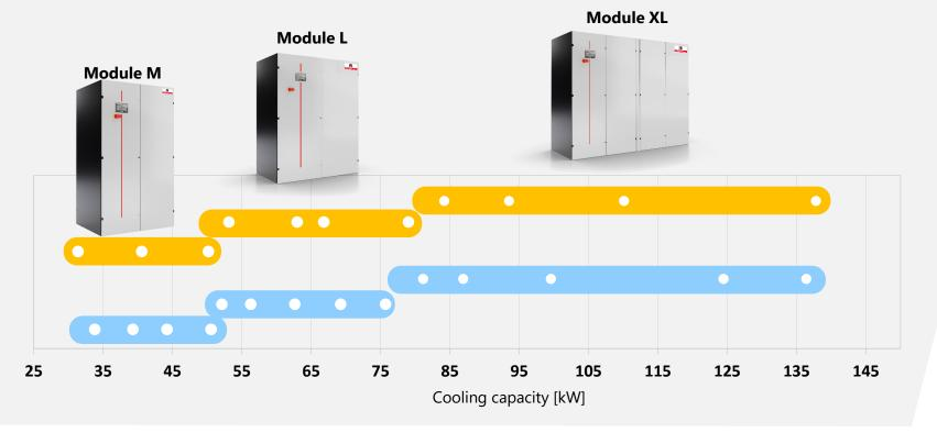
@Return air 30 °C, 35% RH, Condensing Temperature 45 °C
