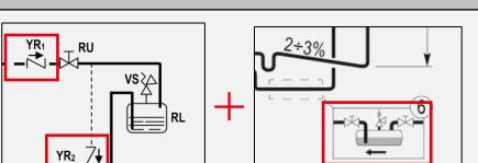
An additional liquid receiver can be requested in addition to the low temperature kit to be installed on the liquid line outside the unit
