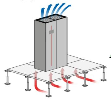
**OVER** air flow delivery and return from the **bottom**. Ideal for data centers with raised floor.
